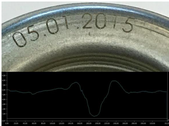
Figure 5: Laser penetration depth limited to 6 \mu\text{m}
