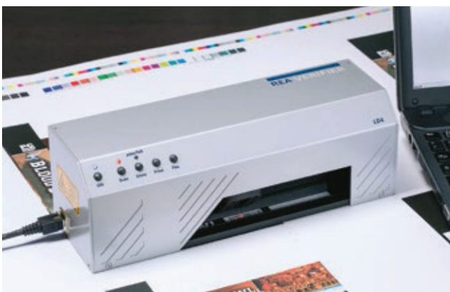
Measuring of barcodes on print sample sheets
