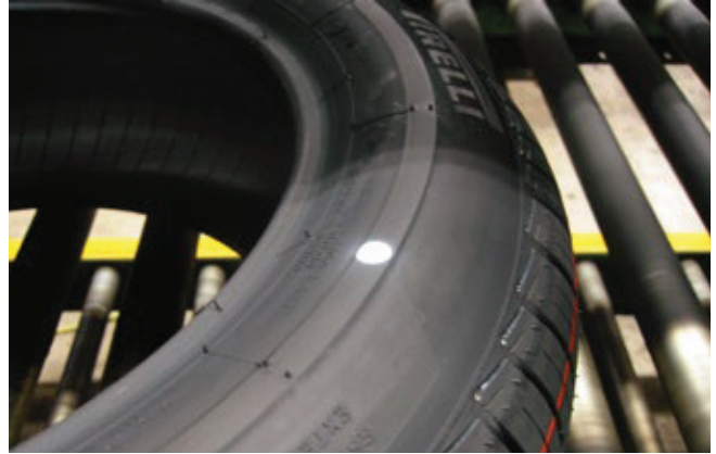
High-point marking on tires
