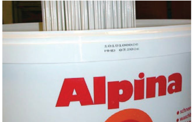
Marking of plastic paint buckets
