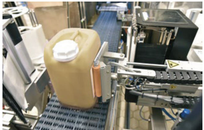
Multi-sided canister labeling
