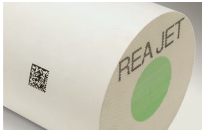
Marking of 2D codes on particle filters
