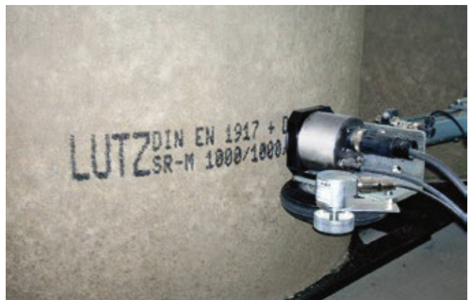
Marking of concrete pipes
