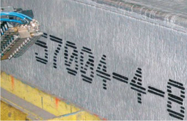
Marking of aluminum ingots
