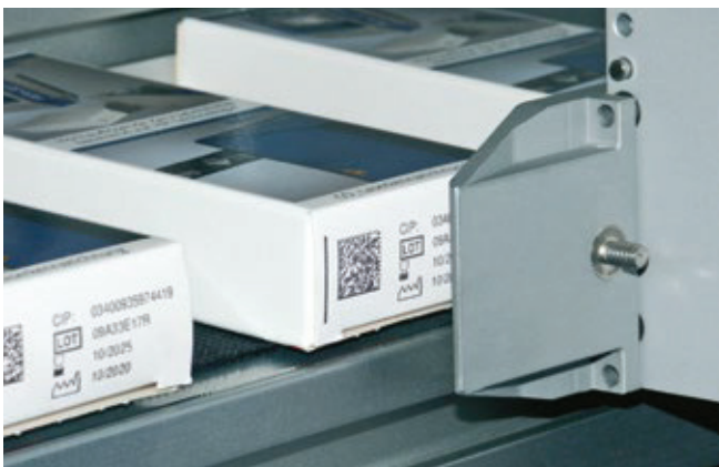
Coding and marking of folding boxes with Data Matrix codes
