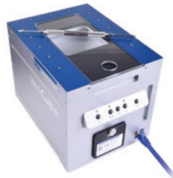
REA VeriCube DPM with diffuse illumination (for UDI code verification)
