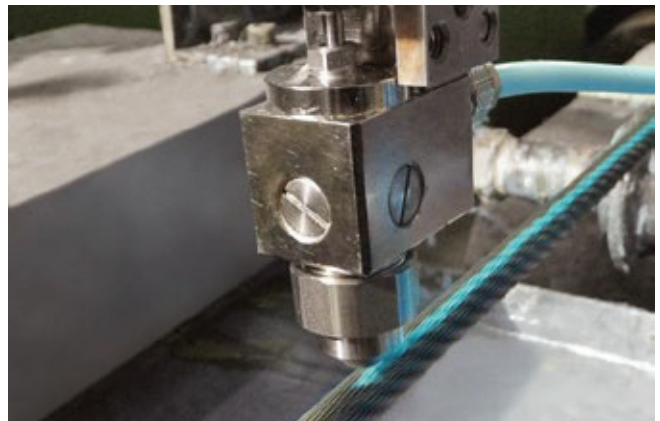
Color marking of wire cables
