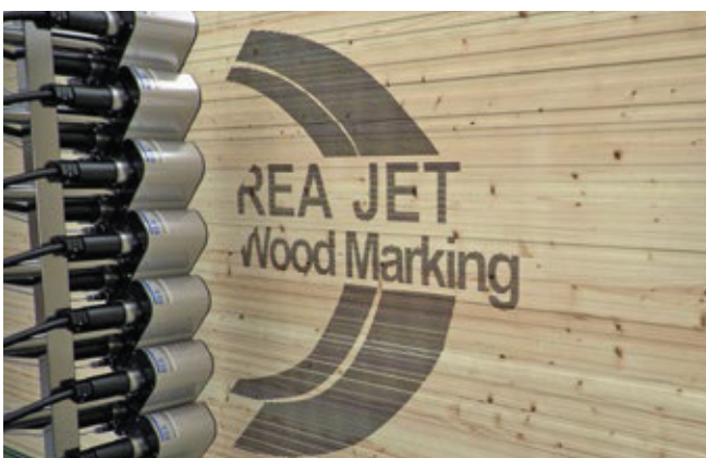
Large marking of logos on stacked boards
