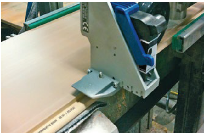
Coding and marking of laminate
