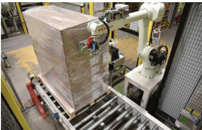
Robot labeling of pallets
