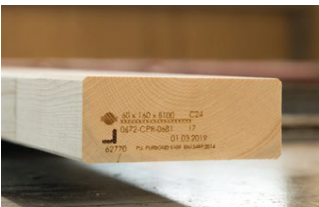
Wood marking with CO 2 laser
