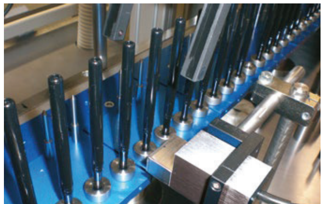
Precise application of oil on plastic parts
