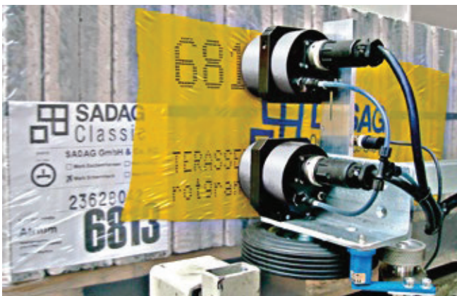
Coding and marking of shrink hoods
