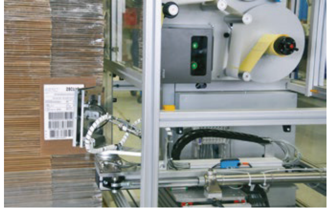
Pallet labeling (one stop for two sides)
