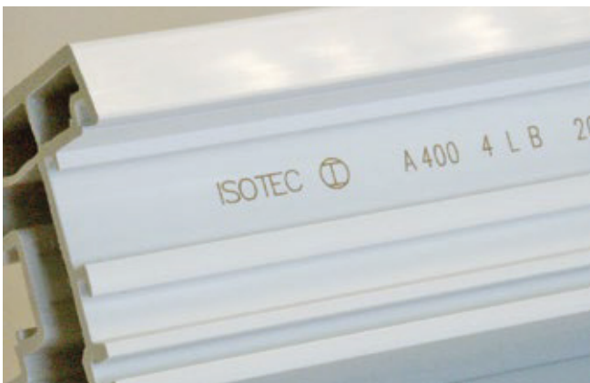
Coding and marking of plastic profiles
