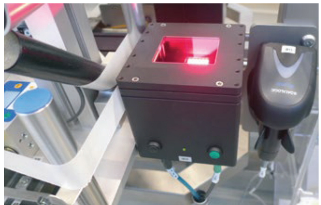
Code verification device integrated into the packaging machine
