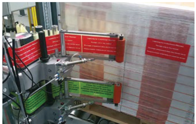
Robot labeling of pallets
