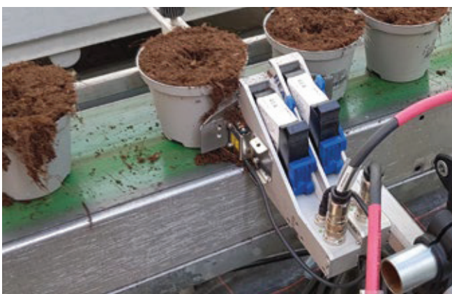
Direct marking with the EU plant passport
