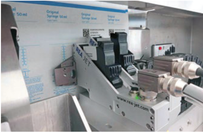
UDI marking of packaging material
