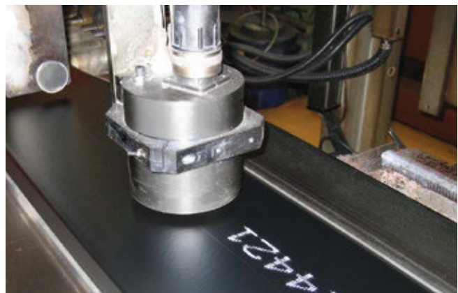
Marking of tread on raw rubber
