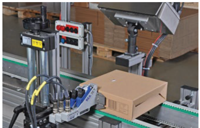
Marking cardboard boxes with barcodes
