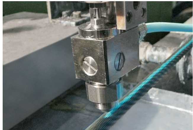
Line marking on steel cables as an assembly aid (swirl marks) for passenger lifts
