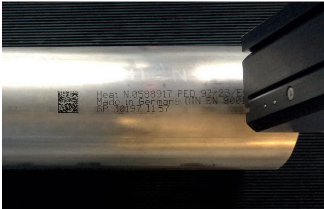
Coding and marking of steel pipes
