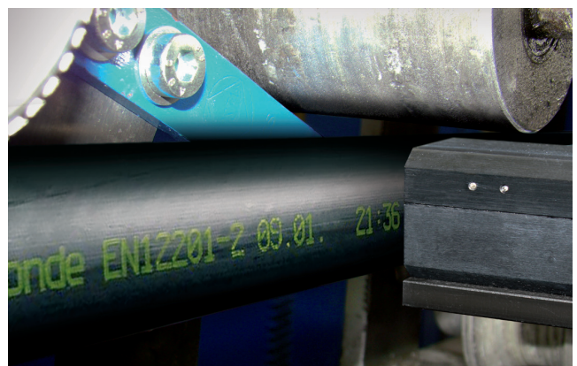
Marking with slightly pigmented ink
