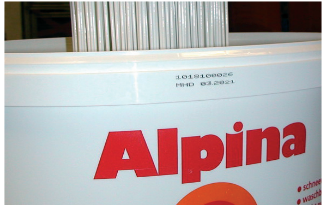
Marking of plastic paint buckets
