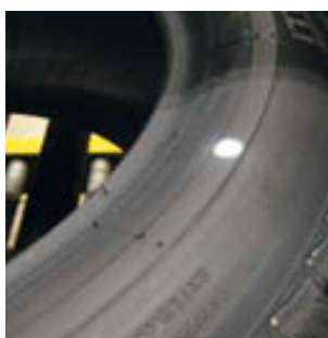
High-point marking on automobile tires
