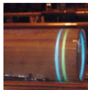
Colored ring marking on steel pipes
